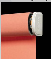
Features: Heavy-duty white plastic covered / metal brackets for face or top fixing, with 53 or 60mm grooved aluminium barrel. Fabric is located in the groove in such a way that, although it cannot be pulled out it may be slid out sideways for repair or replacement. A powerful 240v AC motor is housed within the barrel and is operated by an individual switch. Tear Drop white aluminium bottom bar as standard.
