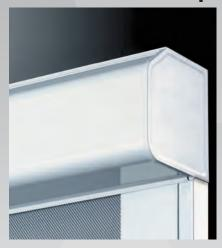
**Features:** C65-85: Aluminium cassette 85 x 97mm with metal end plated and top-fix or face-fix brackets. A heavy duty 240v motor housed within a 53mm barrel to which the fabric is attached. The motor is controlled by a switch which may be surface or flush mounted. Fabric has a 12 x 42mm bottom bar, running in 55mm side channels. Studs fitted at edge of fabric to retain it within side channels. Black or white hardware as standard. C65-115: As C65-85 apart from: cassette size115 x 132mm.
